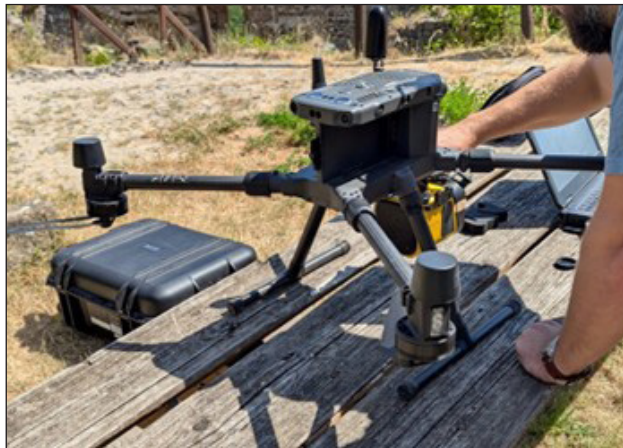
Fig. 6: Aerial Laser Scanning with LiDAR using a drone (Photo: Ábel Hajas)
